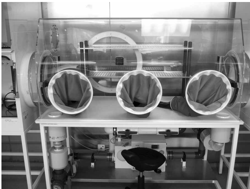
Figure 1. Special digester used in a BSL 4 lab.
