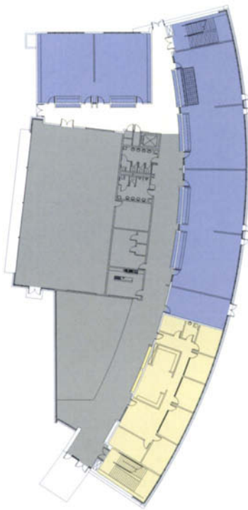
Plan illustrating public spaces located at the perimeter. Concordia International School, Shanghai, China, Perkins Eastman Architects
