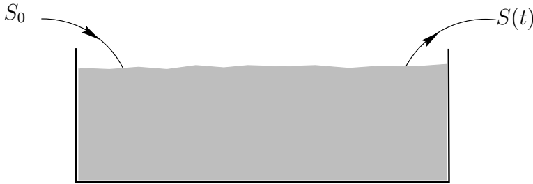
Figure 1.8: THE PRINCIPLE OF THE CHEMOSTAT. AN INFLOW OF PURE NUTRIENT S_0 , WITH RATE R , IS COMPENSATED BY AN OUTFLOW CONTAINING BOTH THE MICRO-ORGANISMS AND THE NUTRIENT AT CONCENTRATION S(t) .
