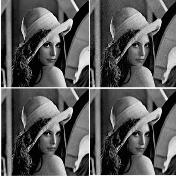
Figure 1: (Top left) Original image and (top right) noisy image 13.95db, (bottom left) denoising by the new algorithm 20.08db and (bottom right) denoising by the original algorithm 19.36db
