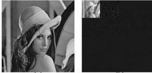
FIGURE 2. An original image with resolution 128 \times 128 , and the two-level wavelet decomposition
