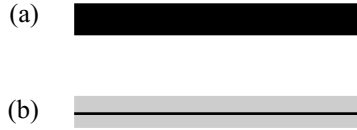
Figure 7.4. The isotropic solid model of graphene (a) contrasts with a structural model (b) in which all the in-plane stiffness comes from the thin central layer (black) and all the bending stiffness comes from the surrounding (grey) material.
