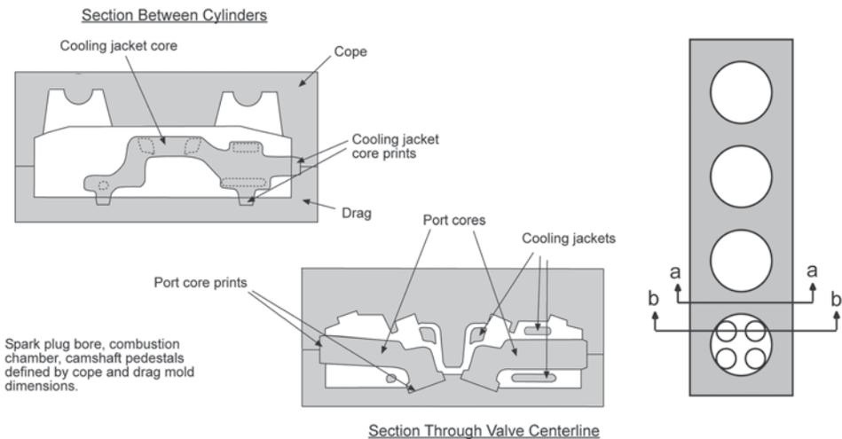
**Fig. 7.4** Schematic depicting cylinder head casting considerations
