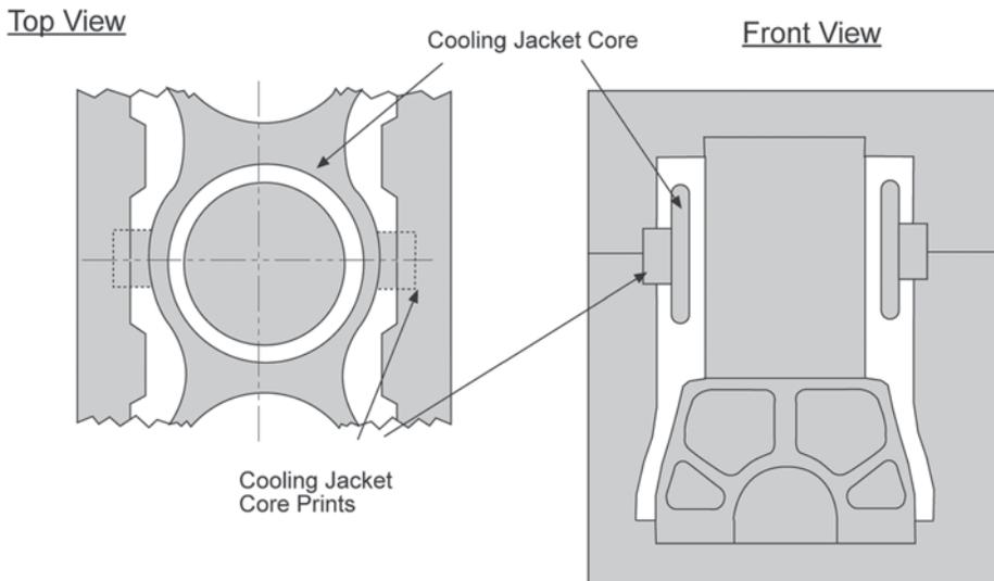
**Fig. 7.7** Closed deck casting schematic
