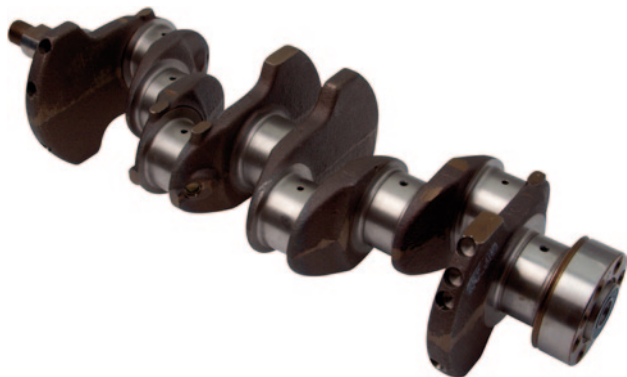
Fig. 16.31 Crankshaft drilling for balance, oil passages
