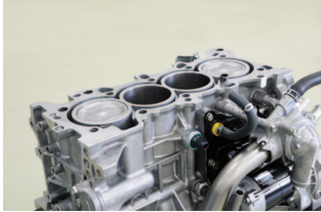
Fig. 7.8 Open deck cylinder block
