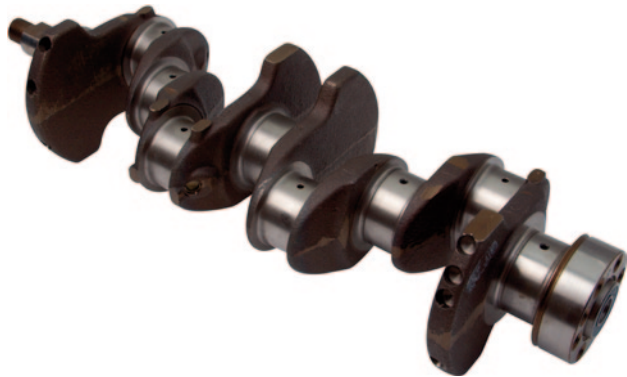
Fig. 16.31 Crankshaft drilling for balance, oil passages
