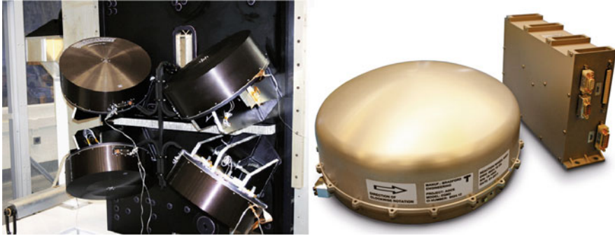
Fig. 6.42 Left: Reaction wheels on Lunar Reconnaissance Orbiter, NASA GSFC (Image: NASA); right: Reaction wheel unit (Image: bradford-space.com)
