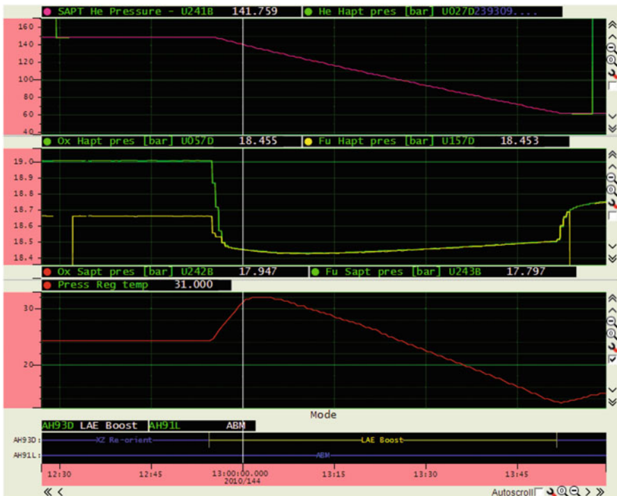
Fig. 6.36 Pressure evolution during AMF2. First plot on top displays the pressure in the helium tank. The second plot shows the pressures in both oxidizer (U057D in green ) and fuel (U157D in yellow ) tanks. The third plot shows the pressure regulator temperature and the last plot at the bottom depicts the state of the AOCS software, showing when the orbit maneuver takes place
