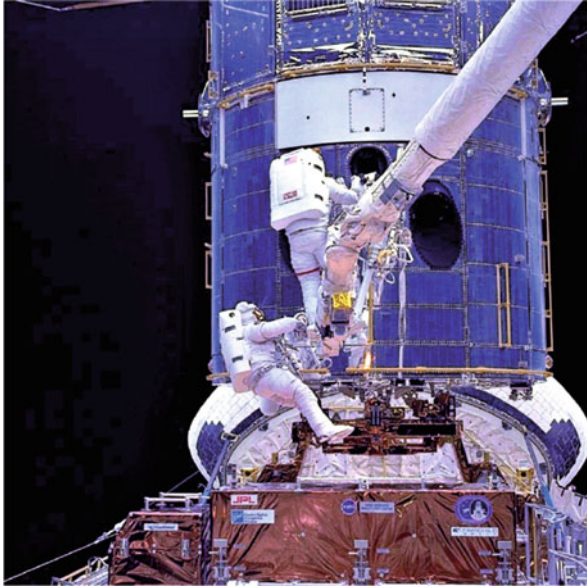
Fig. 7.6 Servicing mission SM1 (STS-61) for Hubble Space Telescope installing corrective optics in December 1993 (credit: NASA)
