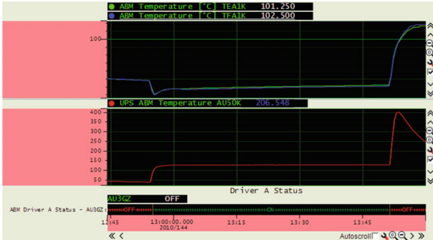
Fig. 6.37 Temperature evolution during AMF2. First plot on top shows the temperature at the inlet of the combustion chamber. The second plot displays the temperature measured close to the combustion chamber. The last plot at the bottom gives the status of the engine valve, showing when the orbit maneuver takes place
