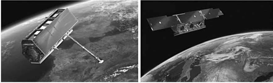
Fig. 6.27 Deployable and undeployable solar arrays. For TerraSAR-X ( left ) the solar panels are mounted on the upper right of the satellite. Since its follower TerraSAR-X 2 ( right ) will have higher power consumption, larger solar arrays are needed. Thus the panels have to be deployed after launch
