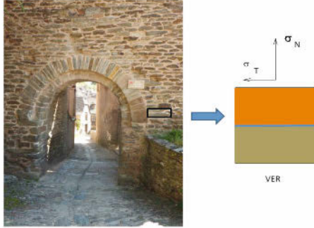
Figure 16. Normal and tangential stress vector components
