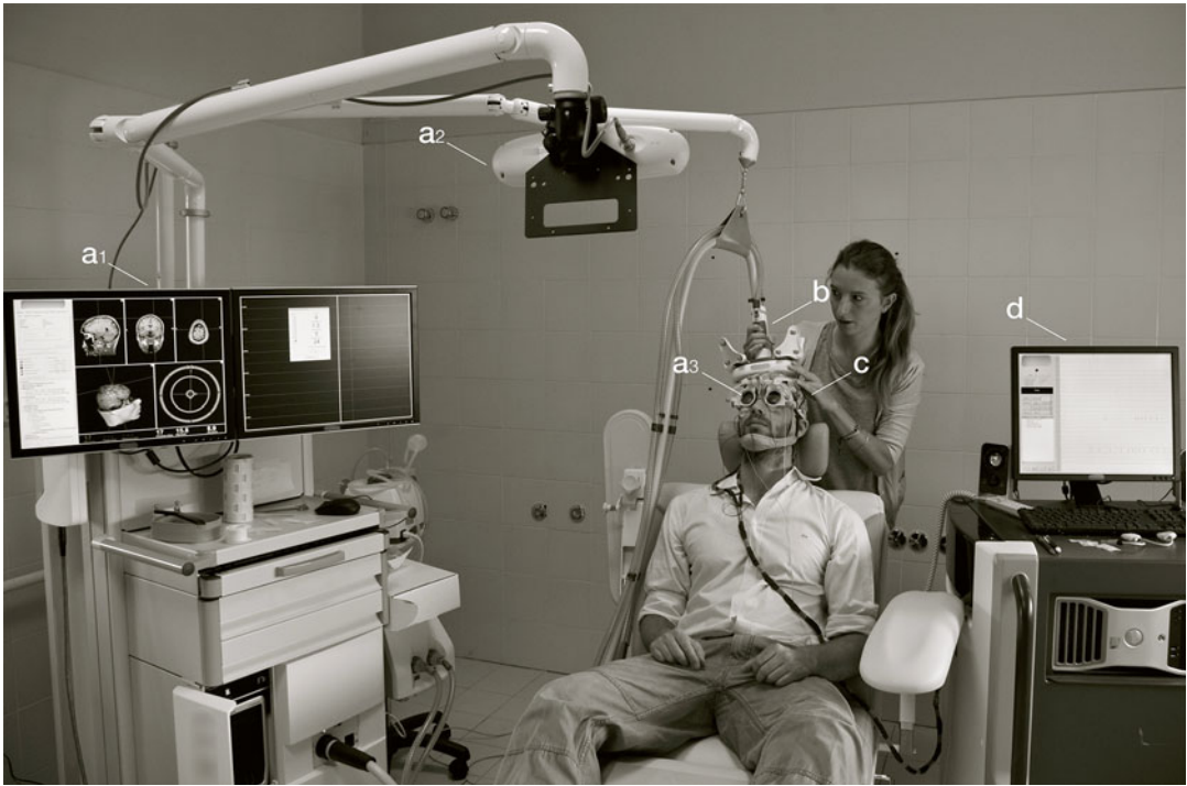
Fig. 10.1 Neuronavigated TMS-EEG system. The neuro-navigation system is composed of a 3D head model and targeting system ( a1 ), an infrared camera ( a2 ), and glasses ( a3 ) that are covered with reflective balls for infrared tracking. The stimulation coil ( b ) is also covered by these reflective balls for accurate localization of the stimulation
