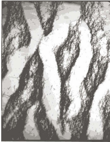
Figure 18. The snake-like veins in the FeSi crystal oriented for single slip cycled at constant low plastic strain amplitude (courtesy of S. Libovický).
