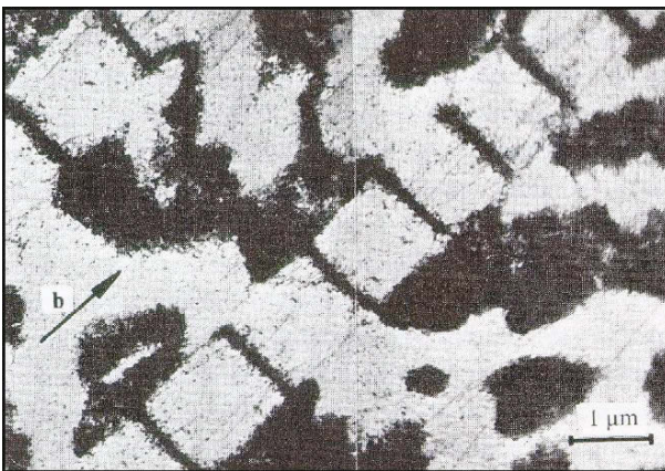
Figure 21. PSB – vein structure (courtesy of H. Mughrabi)
