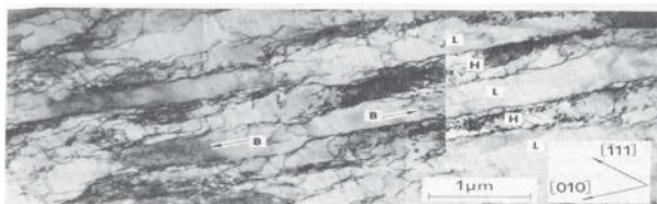
Figure 23. Alternate dislocation slabs in Fe-0.9%Si. There are layers of lower (L) and higher (H) density of secondary dislocations between dislocation sheets. The cross-sections of bundles (incidental boundaries) (B) can be seen in layers of lower density. (courtesy of S.Libovický)
