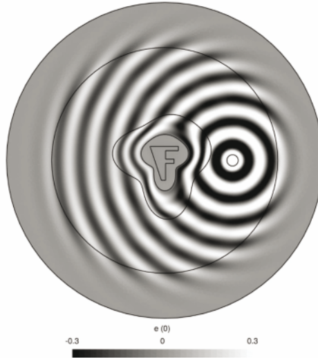
Figure 9. Cloak with a general shape surrounding a F-shaped metallic object in presence of a line electric source generating transverse electric waves. Plot of the real part of the longitudinal magnetic field. (courtesy of A. Nicolet, Institut Fresnel).
