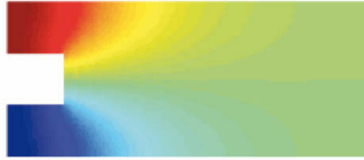
Figure 27. 2D edge resonance in an acoustic waveguide, obtained by symmetry from the trapped mode with a rectangular obstacle.
