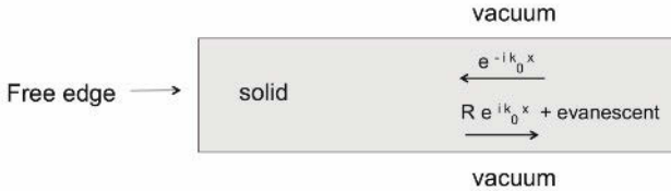
Figure 34. Reflection of the S_0 Lamb mode by a free edge.
