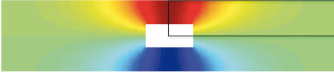
Figure 17. Trapped mode for a symmetric rectangular obstacle in a Neumann waveguide.
