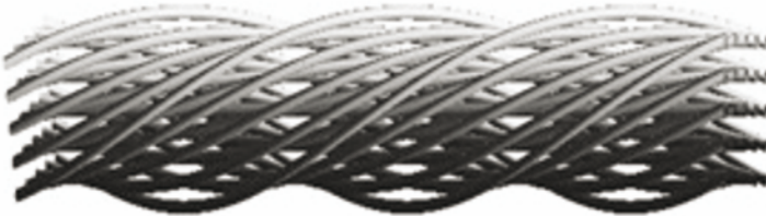
Figure 7. A twisted structure that may be described by the helicoidal coordinates (courtesy of F. Zolla, Institut Fresnel).
