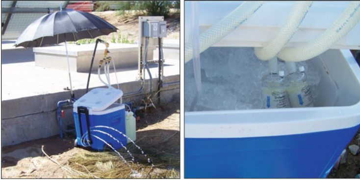
Fig. 12.1 Special sampling precautions to ensure samples remain adequately cooled during prolonged filtration of large volumes of finished water using USEPA Method 1623 filtration equipment. In this example, finished drinking water samples were being filtered for the detection of infectious Cryptosporidium using a cell culture assay (Rochelle et al. 2012). The ambient temperature was 43 °C (110 °F) and samples needed to be kept cool during filtration to prevent inactivation of oocysts (Photos courtesy of J. Hernandez, City of Scottsdale Water Resources Dept. (Arizona, USA))
