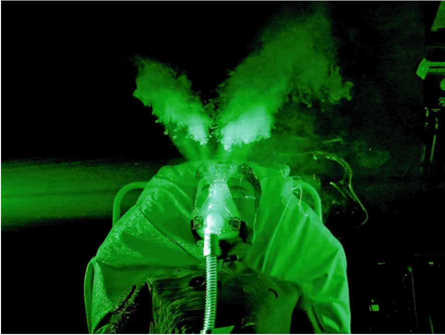
Fig. 2.1 Human patient simulator (HPS) lying at 45^\circ on a bed undergoing noninvasive ventilation via the ResMed Mirage face mask. A laser beam located on the right side of the bed lateral to the human patient simulator illuminates the exhaled air particles leaking from the exhalation ports of the face mask in the coronal plane. A camera was positioned along the sagittal plane at the end of the bed to capture lateral dispersion of exhaled air illuminated by the laser device. Positions of the camera and the laser device would be exchanged when the exhaled air dispersion from the face mask is examined along the sagittal plane
