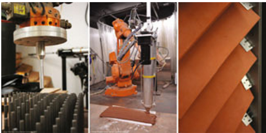
Figure 6 Prototypical manufacturing strategy including robotically actuated variable pin mold, robotic extrusion process, and finished proof-of-concept prototype
