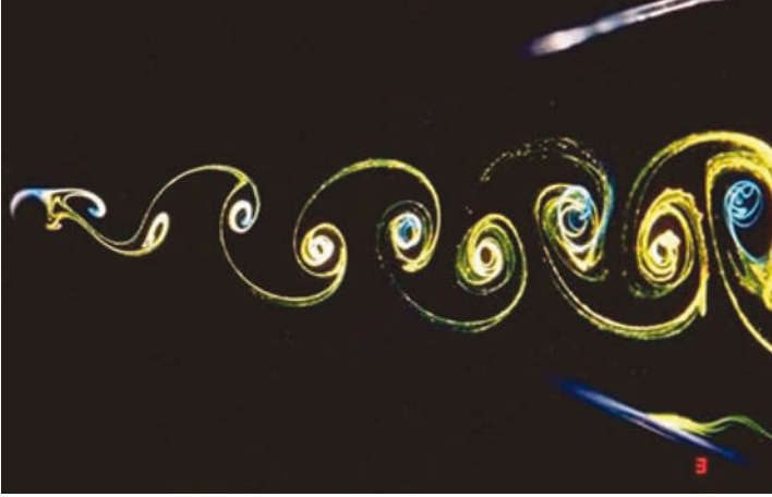
Figure 15. Von Karman vortex street behind a cylinder (copyright Onera, The French Aerospace Lab).
