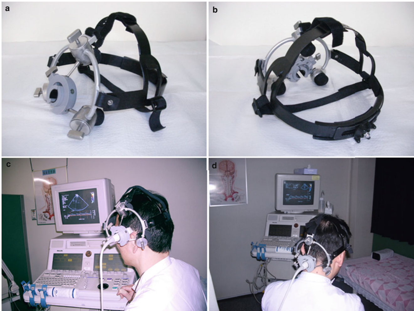
Fig. 1 We have developed and improved the transducer holder (Sonopod) for transcranial color duplex sonography (TCDS) monitoring. (a, b) via both the temporal window (TW; c) and the foraminal window (FW; d)
