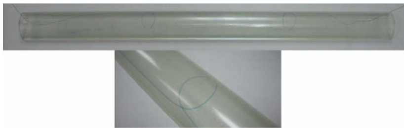
Figure 32. Semicircular tube with embedded fiber optic sensors
