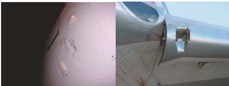
Figure 1. Accidental damage in aircraft structures resulting from ground vehicles
