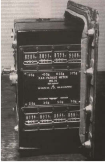
Figure 6. Acceleration exceedance measurement system to be used for loads and fatigue monitoring in aircraft of the Royal Air Force since 1954 (3)
