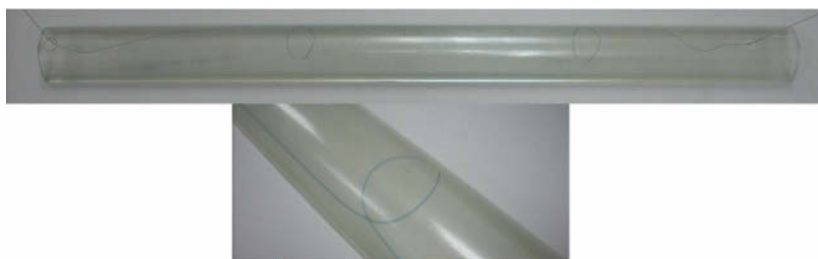
Figure 32. Semicircular tube with embedded fiber optic sensors
