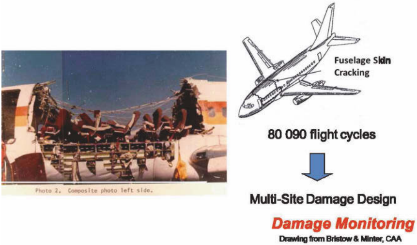
Figure 7. The Aloha Airlines Flight 243 accident as an impact to the ageing aircraft discussion
