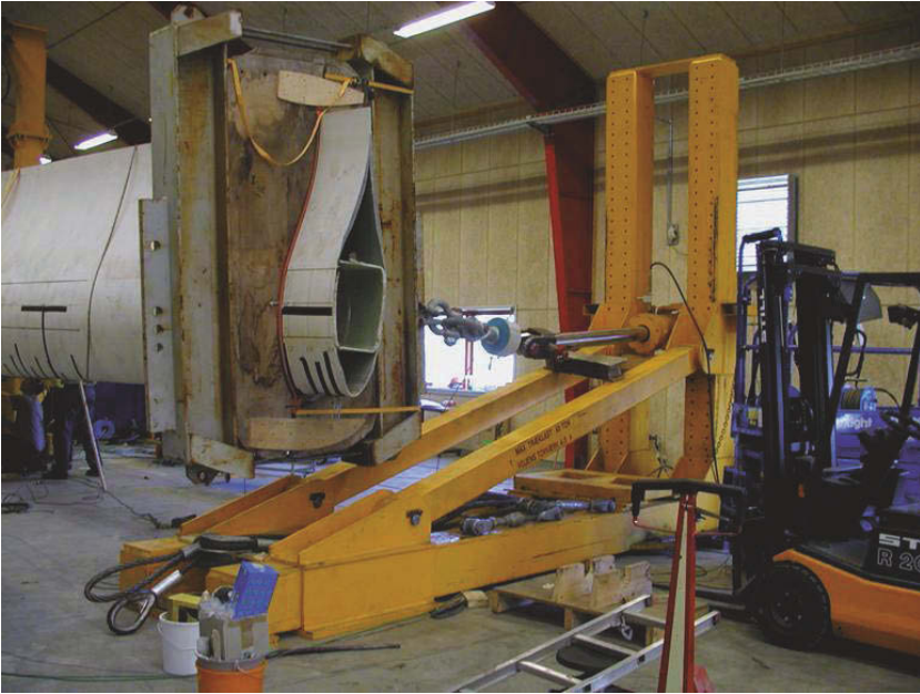
Figure 36. Alternate test configuration with reinforced loading section
