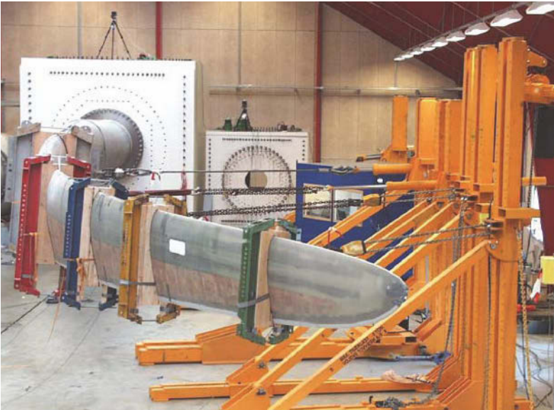
Figure 30. Structural test of a full wind turbine blade.
