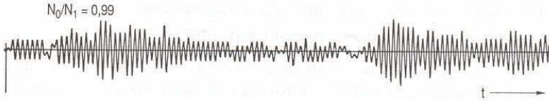
Figure 18. Pseudo-random load sequence generated from a rainflow matrix
