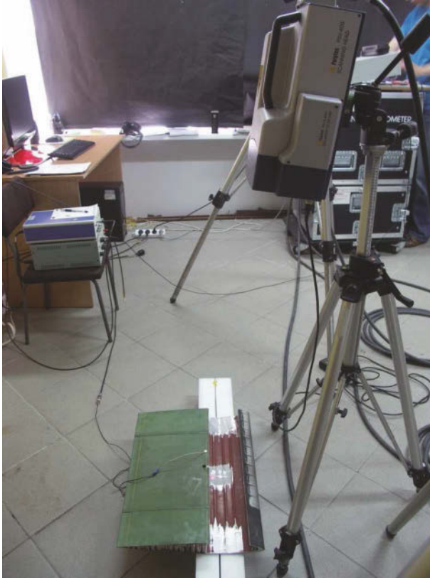
Figure 17. Measurements of elastic wave propagation in the part of helicopter main rotor blade using laser vibrometer
