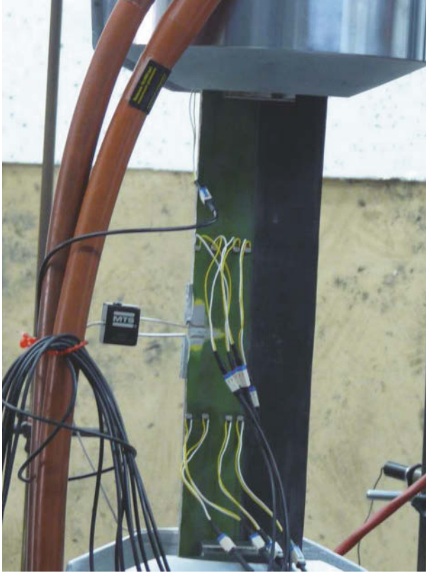
Figure 12. Elastic wave propagation measurements in the part of helicopter main rotor blade during the fatigue tests
