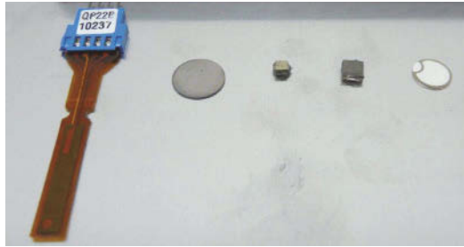
Figure 8. Different types of piezoelectric transducers in authors laboratory; from the left: MIDE QP22B, T216-A4NO-273X Piezo Systems, Inc., Noliac CMAP06 and Noliac CMAP11, Ceramtec Sonox P502 disc
