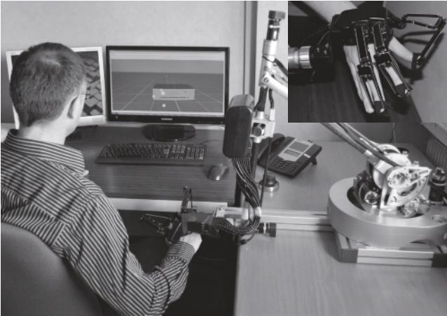
Figure 2. The 3 fingers IHS10 fingertip haptic device.
