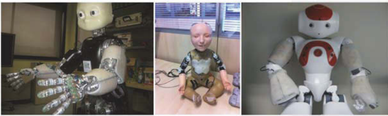
Figure 2. Robots covered with skin patches: iCub, Kaspar and NAO.
