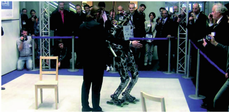
Fig. 10.8 Lola autonomously navigating an unknown environment [20]
