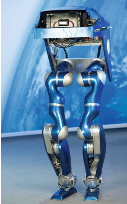
Fig. 8.1 DLR-Biped: a biped walking machine with torque controlled joints
