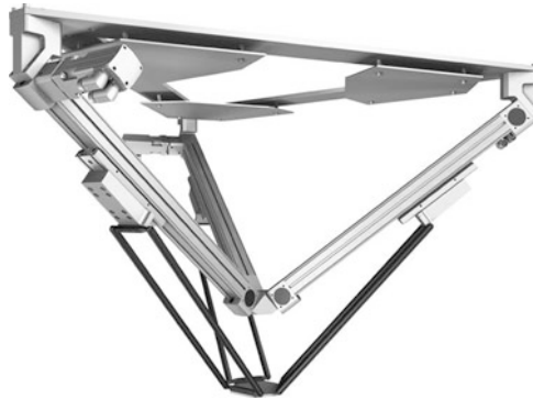
Fig. 12.10 The parameters of a linear drive of a Festo tripod, see also http://www.festo.de , robot are identified. A highly dynamic pick and place motion was chosen to get a good excitation for the measurement
