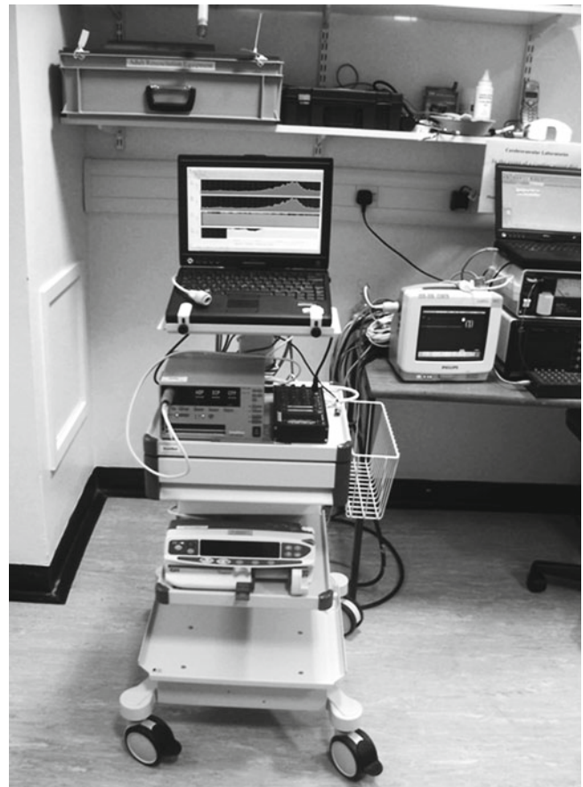
Fig. 1 Infusion test trolley containing a laptop computer running ICM+ software ( upper shelf ), a pressure monitor (Spiegelberg brain pressure monitor) and an analogue-to-digital converter ( middle shelf ), and a syringe infusion pump ( bottom shelf )
