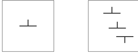
Figure 6. Two strongly different dislocation configurations giving the same \kappa if they are coarse grained for the areas indicated by the boxes.
