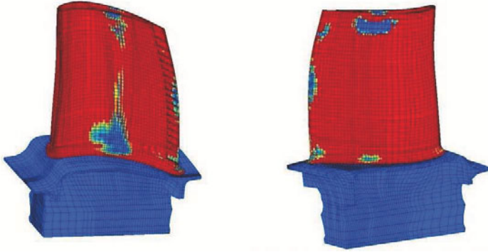
Figure 11. (a) Life prediction on a turbine blade submitted to a thermo-mechanical loading
