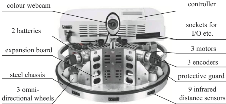
Figure 1. Components of the Festo ROBOTINO
