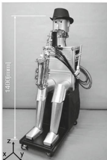
Figure 1. The Waseda Saxophonist Robot No.2 has been developed with 22-DOFs which has improved the design of the mouth and hand mechanisms.
