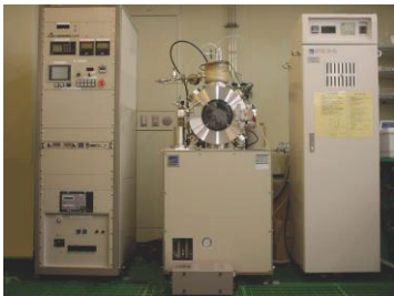
Figure 1. Fast Atom Beam(FAB) manufacturing machine
