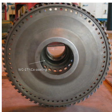
Fig. 1.39 WC–Co coating the internal coating of stage III disc of in aircraft engine
