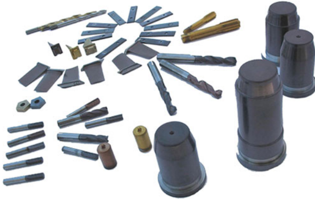
Fig. 2.22 Images of several components coated with nanocomposite film (Dextron Research Ltd., Russia)
