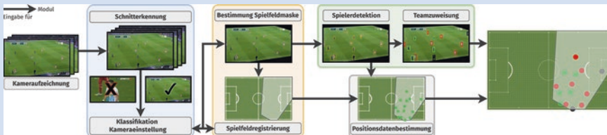
Fig. 4.5.1 Processing pipeline for position data extraction from videos (Theiner et al., 2022)
