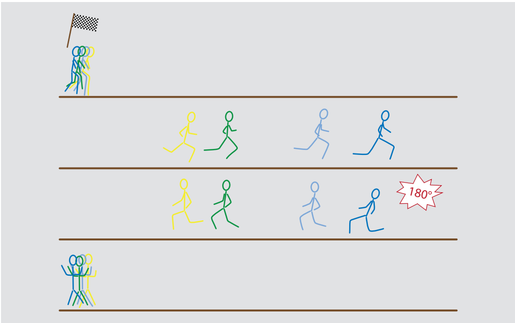
Fig. 7.9 The refocusing impulse using the example of a group of runners: if all runners remain constant in their pace, they will arrive together at the start again when they turn around at the same time, e.g. 30 s later
