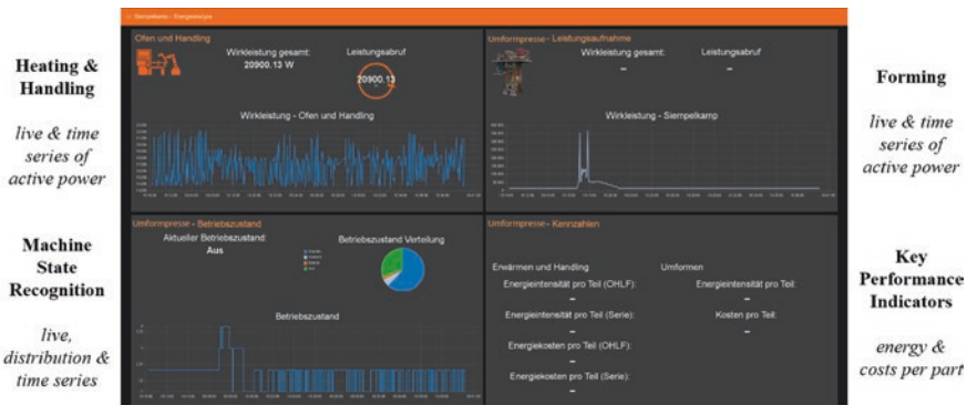
Fig. 4.6 Forming press energy dashboard at the Open Hybrid LabFactory (picture: Siempelkamp)
