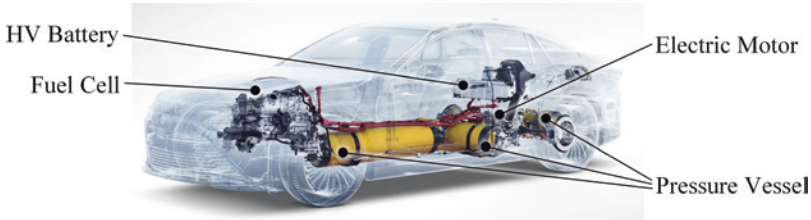
Fig. 2. State-of-the-art fuel cell electric vehicle (FCEV) with 70 MPa tank technology, illustrated by the example of a Toyota Mirai 2 [9]
