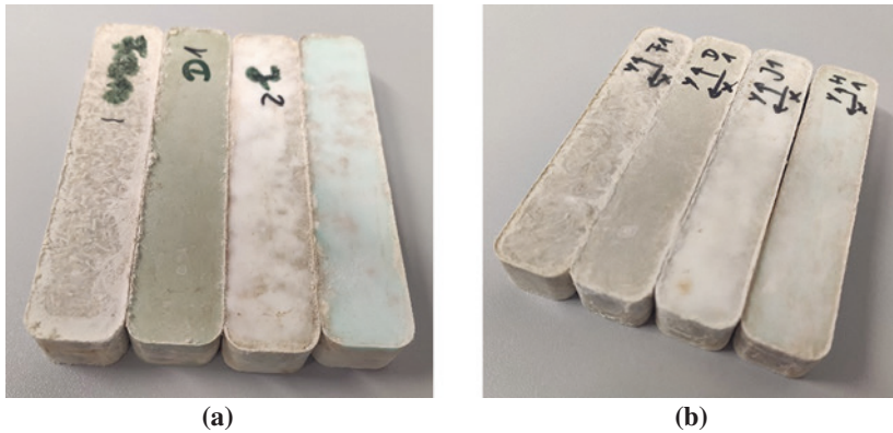
Fig. 2 Compression-molded cores of series A – from left to right: A0, A1, A3, A2 (a), and series B – from left to right: B0, B1, B3, B2 (b)
