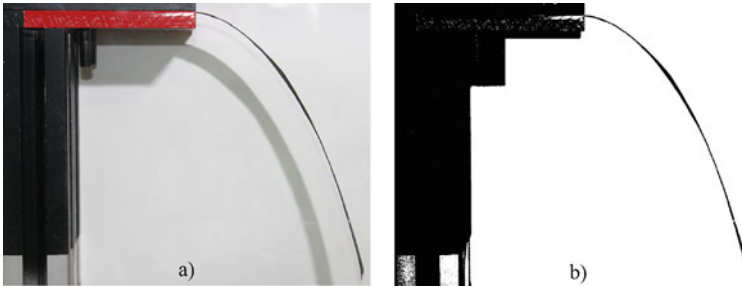
Fig. 2. Images inside the oven: a) original, b) black and white transformation
