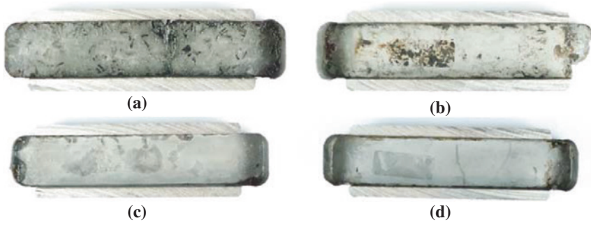
Fig. 6 Surfaces of the cast specimens. (a) Specimen A0 corresponding to the non-coated salt cores made with fibers of 3 mm length. Fiber infiltrations and residuals of burnt fibers are visible. (b) Specimen B0 corresponding to the non-coated salt cores made with fibers of 15 mm length. Only residuals from burnt fibers are observed, no relevant infiltration with melt takes place. (c) Specimen A2 corresponding to a coated salt core made with fibers of 3 mm length. A clean surface was achieved. (d) Specimen B1 corresponding to a coated salt core made with fibers of 15 mm length. The coating also prevents the adhesion of fiber residuals to the cast surface
