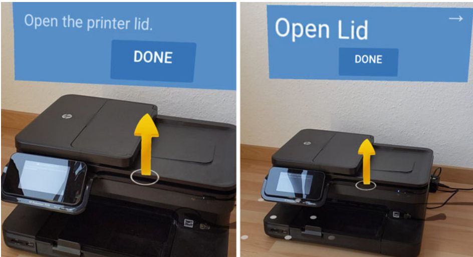
Fig. 6 Distance-based adaptation: When the user moves away from the printer, the level of detail is decreased while the text size is increased
