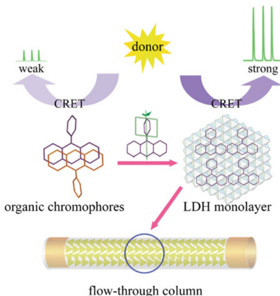
Fig. 10.10 Schematic illustration of universal CL flow device. Reprinted with permission from Ref. [76]. Copyright 2013 American Chemical Society
