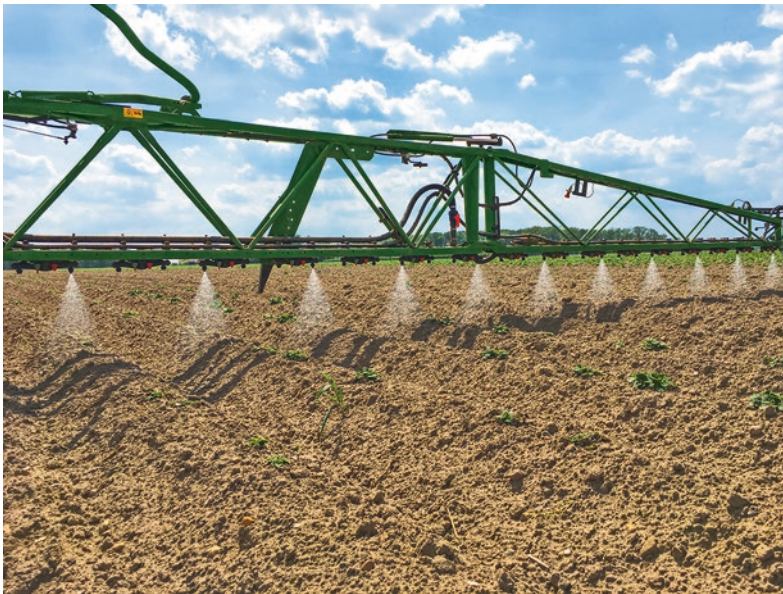
■ Fig. 4.20 Band spraying with the field sprayer and AmaSelect Row
