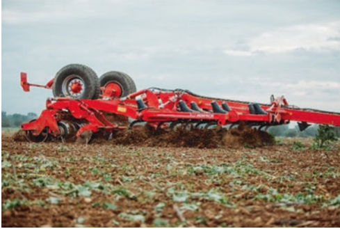
■ Fig. 4.7 HORSCH Tiger 4AS with SteelFlex Packer working in an intermediate crop
