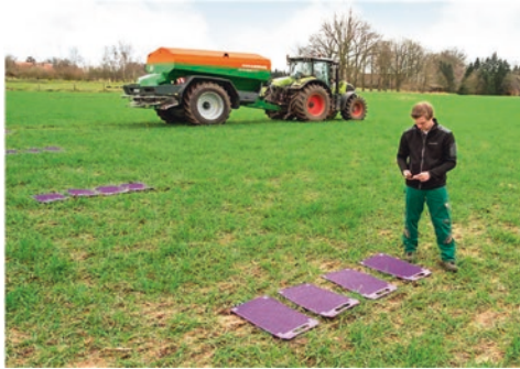
■ Fig. 4.12 Checking lateral distribution with AMAZONE Easy Check [Ama20b]
