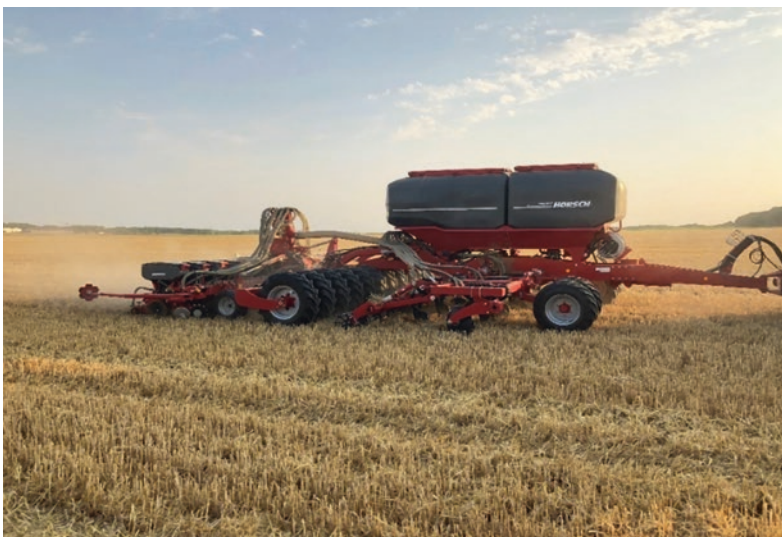
■ Fig. 4.9 HORSCH Focus 6 TD in rapeseed sowing + deep fertilization
