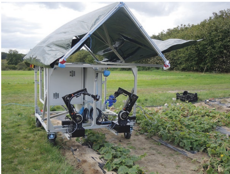
■ Fig. 5.6 Selective pickling cucumber harvest prototype “CATCH” [FRA18] (Photo: ATB)
