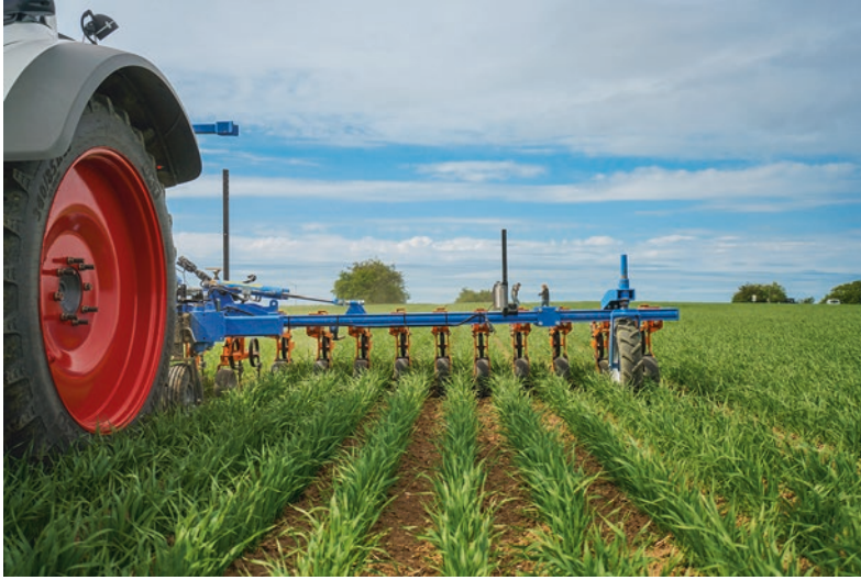
■ Fig. 4.19 Modern hoeing technology with camera guidance
