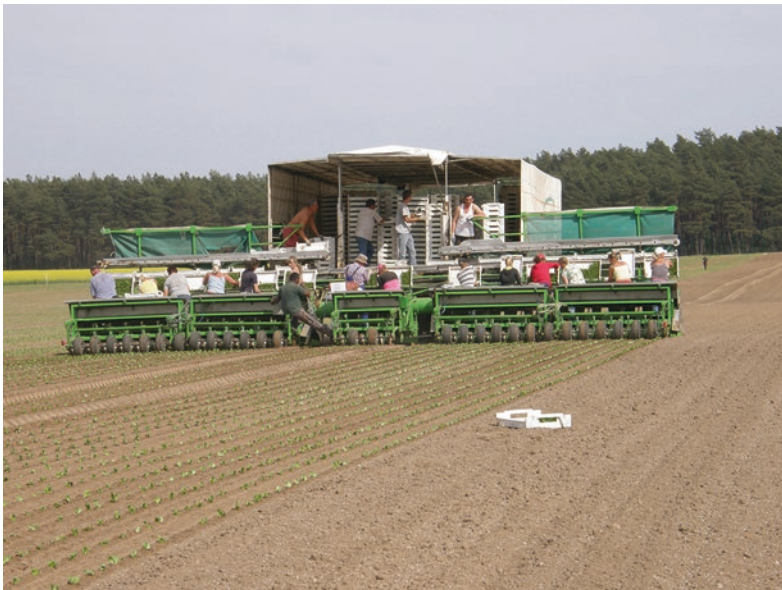
■ Fig. 5.5 12-m wide transplanter for soil press pots (Photo: Geyer)
