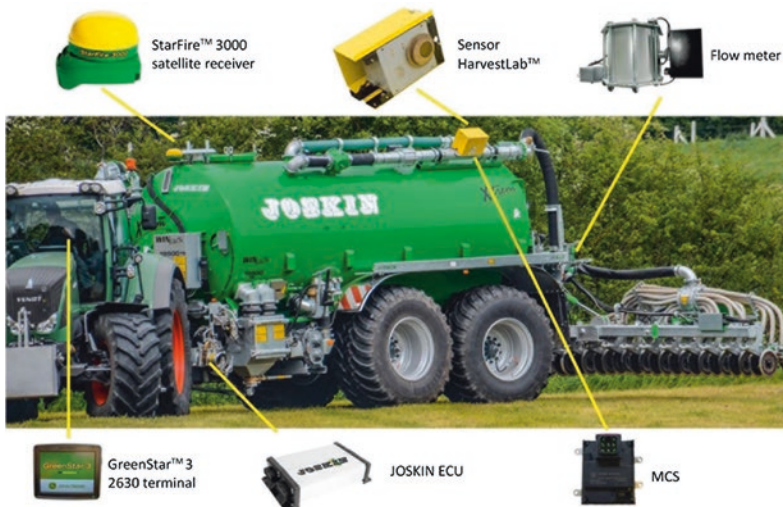
Fig. 4.17 System components of JOHN DEERE Manure Sensing [Jos20]
