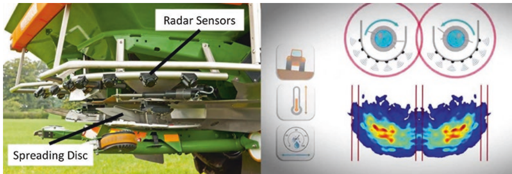
■ Fig. 4.11 Spread pattern monitoring with AMAZONE ARGUS TWIN [Ama20a]
