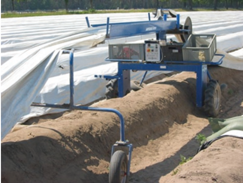
■ Fig. 5.7 Single-row harvesting aid with electric drive (Photo: Geyer)
