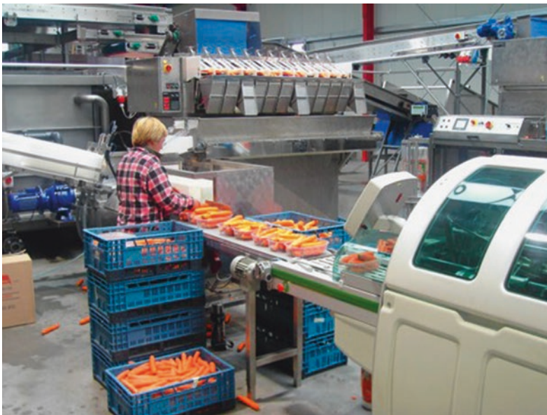
■ Fig. 5.8 Preparation of washing carrots with packing machine and multihead weigher in the background (Photo: Geyer)
