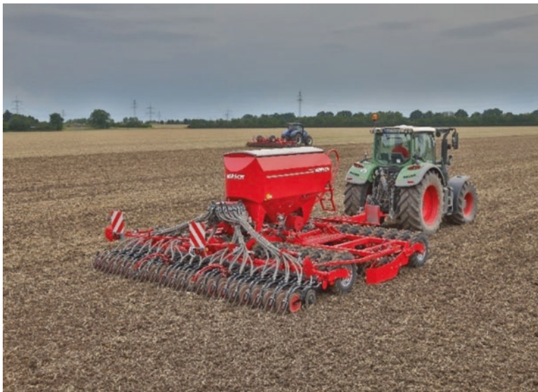
■ Fig. 4.8 HORSCH Pronto 6 DC in grain sowing with variable seed rate
