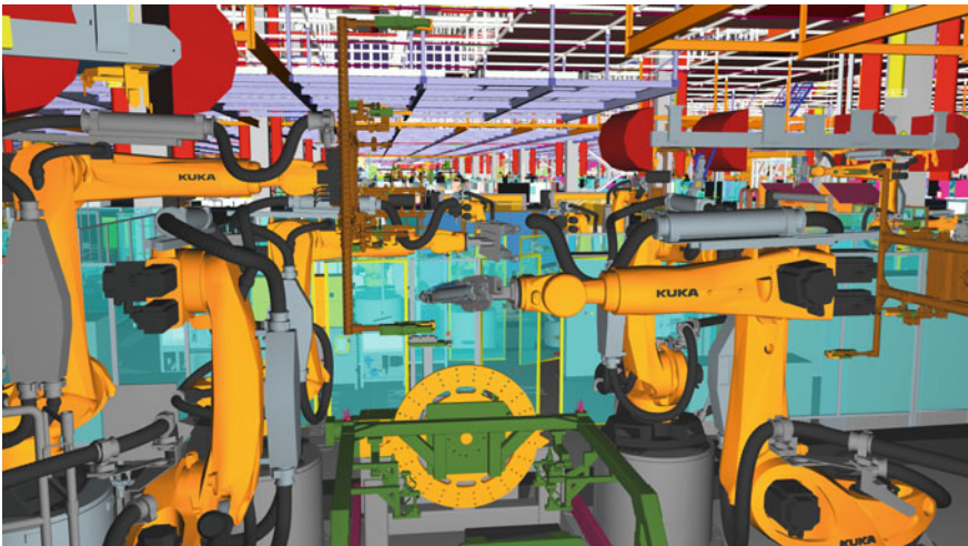
Fig. 15.10 Extract from a 3D model of a robot cell in BIW production [5]
