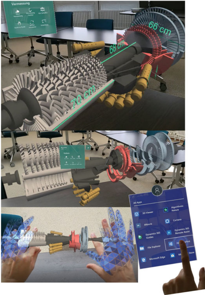
Fig. 14.7 Interactive AR prototype as part of a digital conference room review (example of an aero engine, courtesy by Rolls-Royce)
