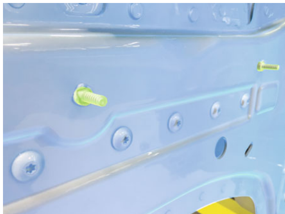
Fig. 14.4 AR based visual inspection of the physical member floor side with its digital product data based on the TWYN system of Visometry GmbH. (Source Porsche Leipzig GmbH)
