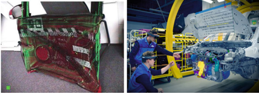
Fig. 14.3 Leftside superposition of a crashed door with the crash simulation result [7]. Rightside augmentation of the virtual engine compartment with the real body-in-white for product validation. (Source BMW Group)
