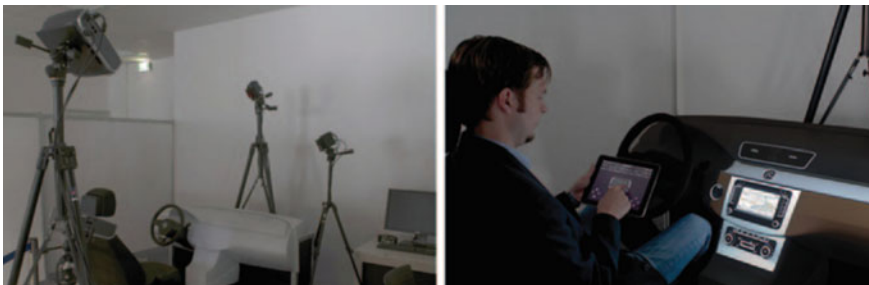
Fig. 14.13 Projection of the cockpit texture onto a rapid prototyped design mock-up apart of the automotive interior design process [13]
