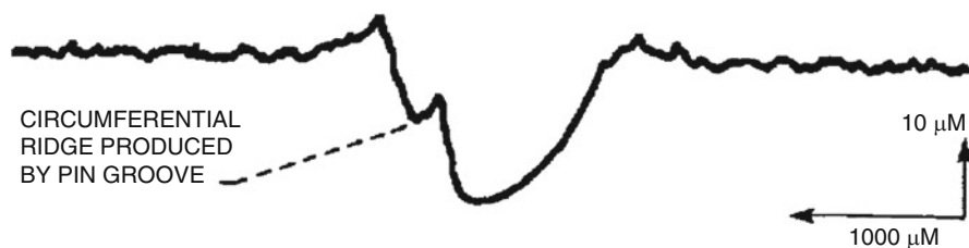
Fig. 4.9 Surface profile of the sliding contact areas [30]
