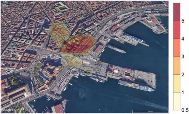
Fig. 2 CFD—distribution of SO 2 concentration [ \mu\text{g}/\text{m}^3 ] in the calculation domain at ground level
