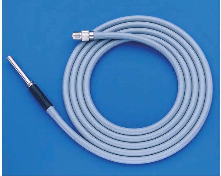
■ Fig. 4.24 Fibre optic cable. (From: Carus (2014))
