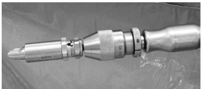
■ Fig. 4.64 Jacob's chuck with trepan clamped in a drilling machine. (Photo by Margret Liehn)
