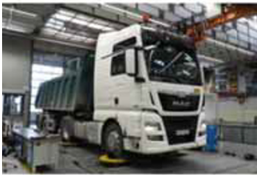
Fig. 2. Physical (left) and virtual (right) hydraulic test rig for trucks and busses. The virtual test rig uses a multibody simulation model with a flexible frame structure
