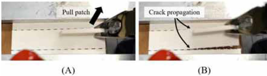
Fig. 3. (A) Pulling of FDM-printed ABS patch with pliers; (B) Initiation and propagation of crack along predetermined, perforated breaking line.
