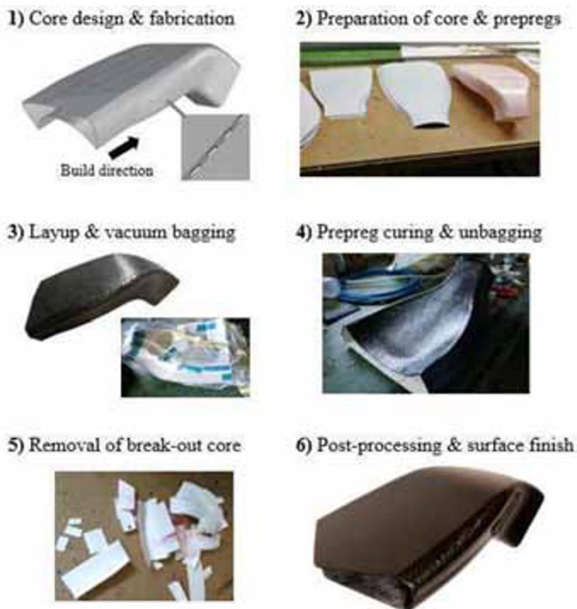
Fig. 7. Visualization of production steps of CFRP flow intake using a break-out core that is fabricated out of ABS using FDM, prepared with release film, used for layup and curing of prepreg material, and removed after composite processing through integrated breaking lines.
