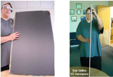
Fig. 5. Double-Double designs using thin plies don't warp and face increased strength
