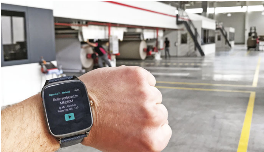
Fig. 5 Exemplary process-based user interface in a corrugation plant
