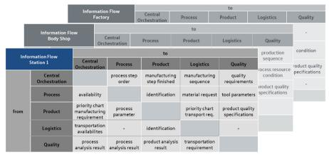
Fig. 1. Interface Matrix for the material flow driven interaction of entities and their information flow on system and station level
