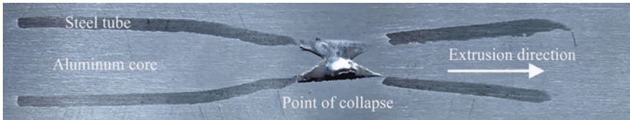
Fig. 1. Failure at the co-extrusion of aluminum with a steel tube
