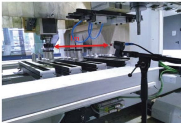
Fig. 2. Measurement of the sound pressure level.
