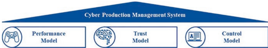
Fig. 2. Required models for the design of cyber production management systems
