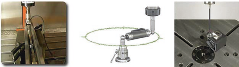
Fig. 2. Rapid test for accuracy: left: comparison scale, middle: circular test with DBB, right: rapid rotatory axis test with AxiSet™ CheckUp
