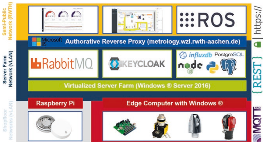
Fig. 3. IoP testbed infrastructure used at the laboratory of the authors comprising sensors, data bases and analysis tools and responsive user interfaces in different network tiers. The copyright of reused logos and device photos remains among their authors.
