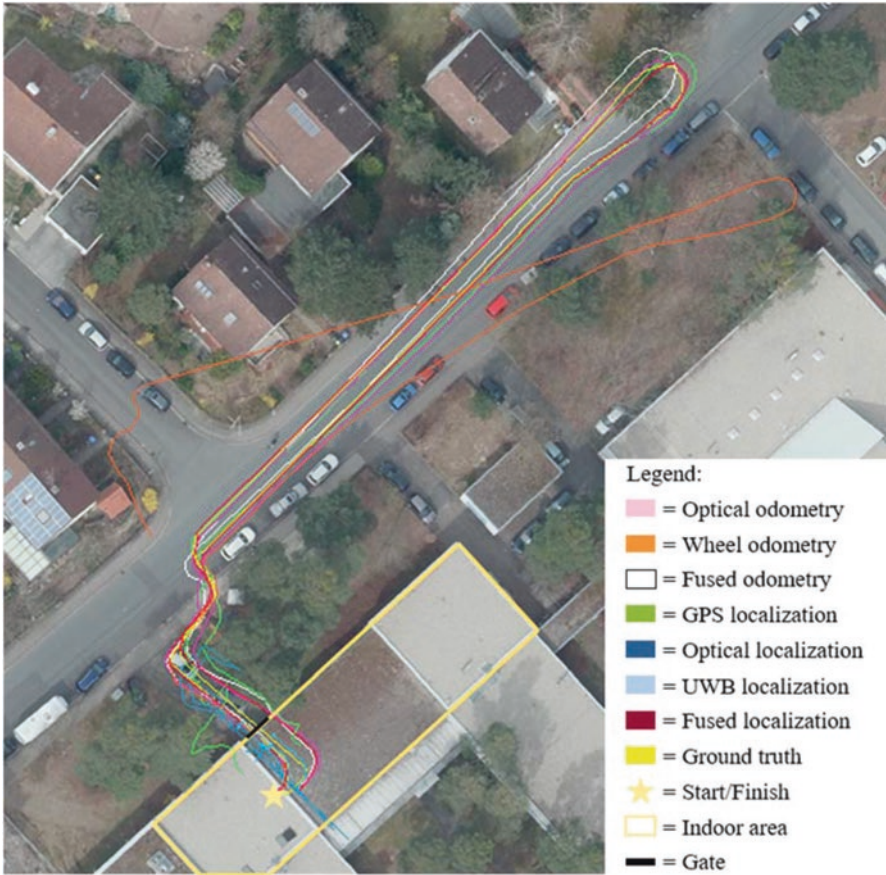
Fig. 3. Test environment and calculated trajectories based on cost-efficient sensor data (Background © Stadt Erlangen/ © Hansa Luftbild AG, CC BY-4.0, [19])
