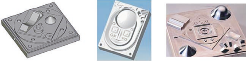
Fig. 1. Left: NCG-HSC test workpiece 2004, middle: NCG-5-axis test workpiece 2005, right: NCG-5-axis test workpiece for microchip removal 2007
