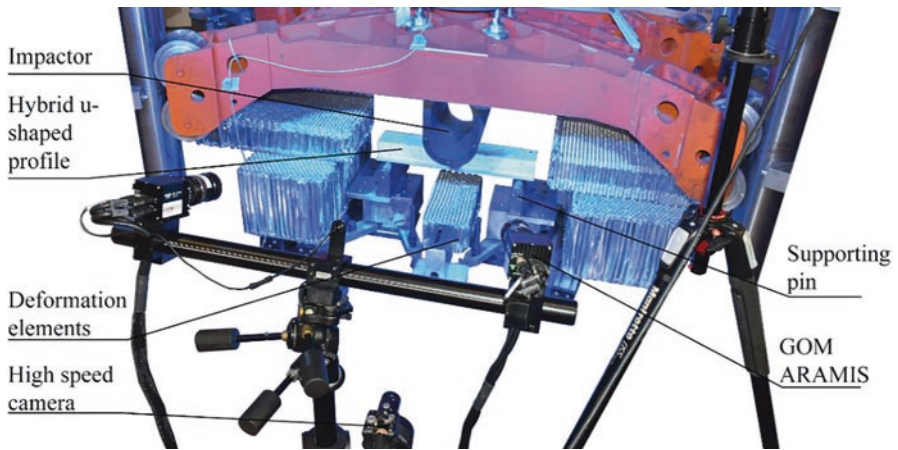
Fig. 4. Setup for the dynamic testing of u-shaped profiles manufactured in an integrated process
