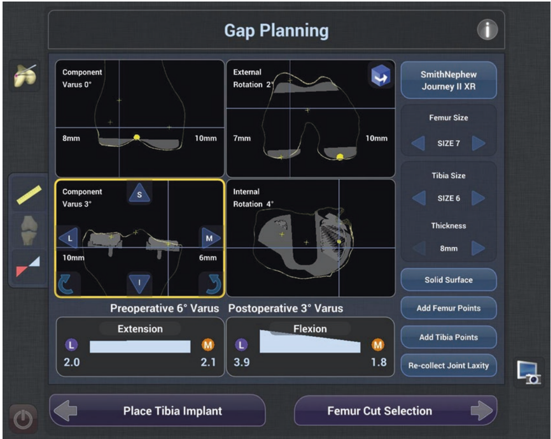
Fig. 3.18 Individual KA plan for a bi-cruciate retaining implant. In contrast to classical CR/PS or medial pivot TKA designs, the gaps have to be more loose
