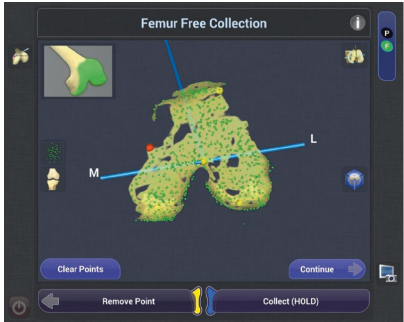
Fig. 3.16 The software calculates an individual 3D reconstruction of the patients knee at the beginning of the surgery
