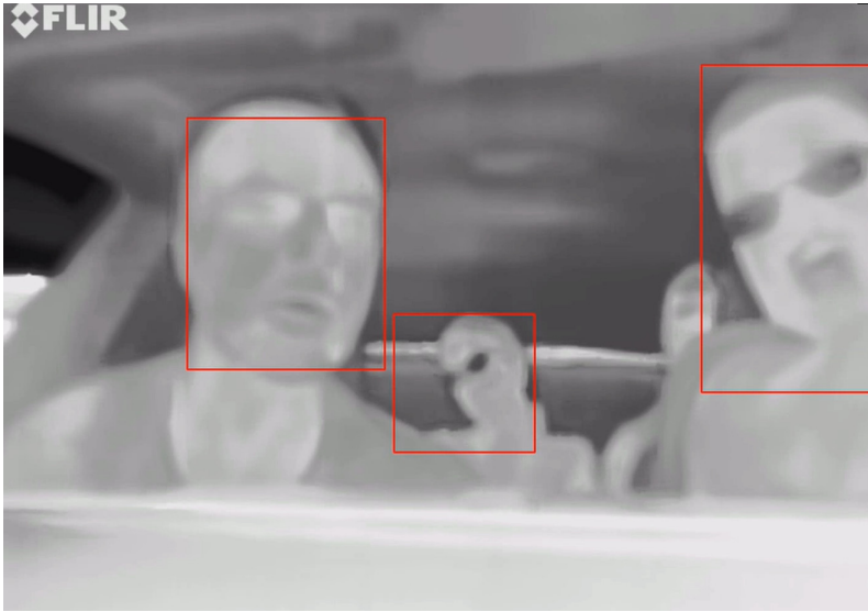
Fig. 7. Face detection using SSD method in an image from thermal camera (Raspberry Pi NoIR Camera HD v2). Detected faces locations are marked with red boxes. (Color figure online)
