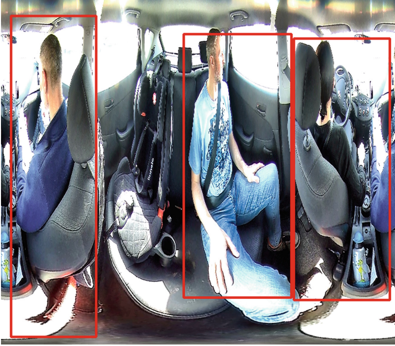
Fig. 8. Person detection using YOLO method in an image from 360° camera (SJCAM SJ360). Detected figures locations are marked with red boxes. (Color figure online)
