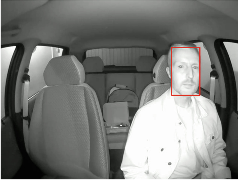
Fig. 6. Face detection using SSD method in an image from infrared light wide angle camera (Waveshare HD Night Vision E OV5647) with LED illumination. Detected face location is marked with red box. (Color figure online)
